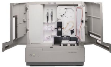
Capillary Sequence (16 Capillary)
